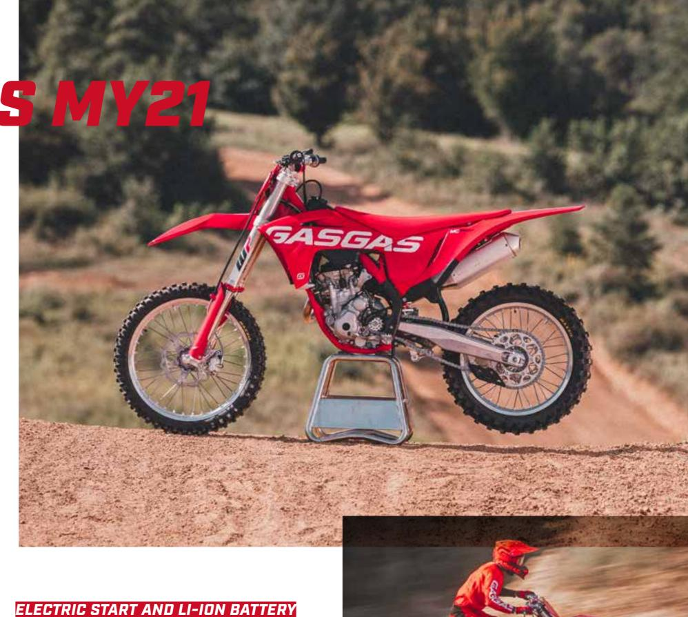
No need to kick, kick, kick! All GASGAS Motocross bikes are fitted with an electric starter as standard. Saving time at the start of a day when a motor's cold, or near the end of a race when the motor's hot, with the simple press of a button both the MC 250F and the MC 450F fire into life. Using a lightweight Li-lon 2.0Ah battery together with a robust starter motor from Mitsuba and a reliable starter drive guarantees reliable starting. Always.
