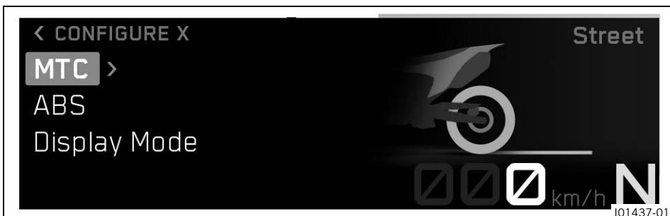
In the combination instrument, the motorcycle traction control can be switched on or off via the **MTC** submenu.
