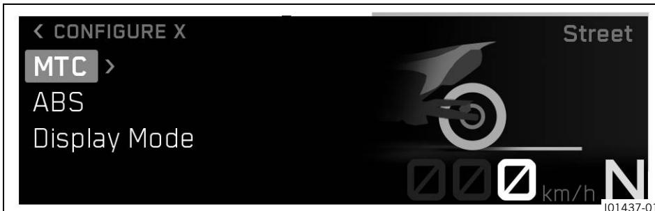
The motorcycle traction control (**cornering MTC**) lowers the engine torque in case of loss of traction in the rear wheel. Depending on the riding mode, different amounts of slip are allowed when the traction control is activated.
