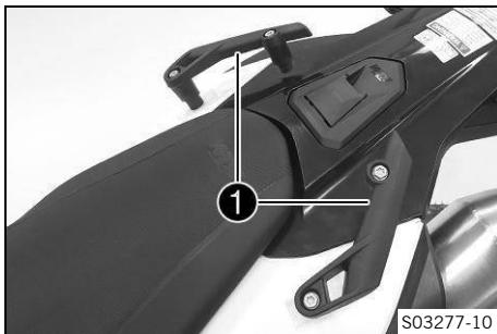
The grab handles 1 are used for moving the motorcycle around. If you carry a passenger, the passenger can hold onto the grab handles during the trip.
