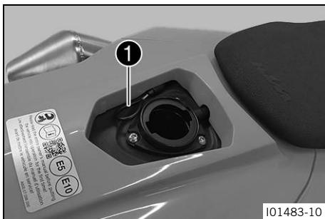
The loop 1 for unlocking the seat is located under the fuel tank cap.
