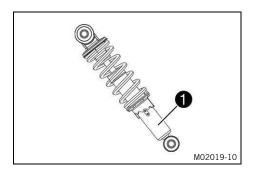
Shock absorber article number **1** is stamped on the bottom of the shock absorber.
