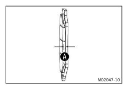
Check all brake pads on both brake calipers for their lining thickness (A).
