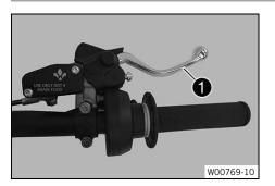
The hand brake lever of the front brake system **1** is attached to the handlebar on the right.
