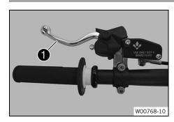
The hand brake lever of the rear brake system 1 is attached to the handlebar on the left.
