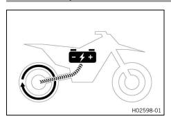
The LV traction battery is charged by the electric engine in ride mode 3 and 6 (p. 22) when the throttle grip is closed beyond the basic position in overrun.
