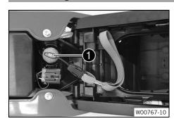
The holder for the gray magnetic switch 1 is located under the seat
