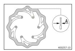
Check the brake disc thickness of the front and rear brake disc at several places on the disc to see if they conform to measurement A.
