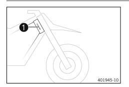
The vehicle identification number **1** is stamped on the right-hand side of the steering head.
