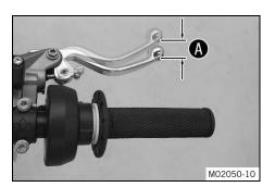
Push the handbrake lever forwards and check play
