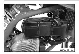
The On/Off button **1** is located on the right side of the LV traction battery.
