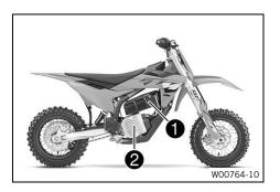
The LV traction battery **1** and the electric motor **2** are aircooled.
