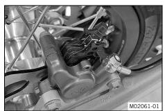
Put the new brake lining in position.
