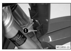
Position the fender with drill holes 1 in the holding lugs on the start number plate.
