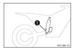
The shock absorber article number **1** is stamped on the bottom of the shock absorber toward the right-hand side.
