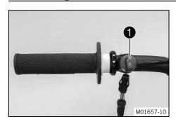
The holder for the red magnetic switch **1** is located on the left side of the handlebar.
