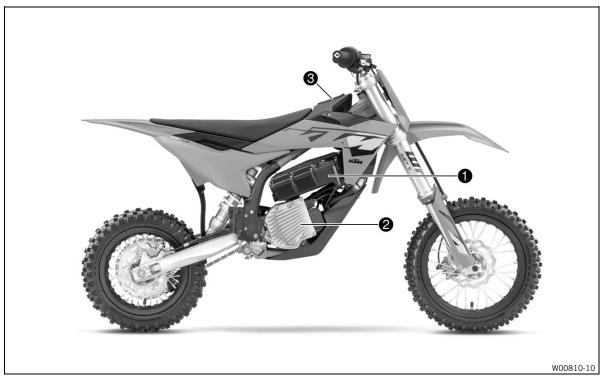
A rechargeable lithium-ion battery 1 (LV traction battery) is installed in the vehicle.
