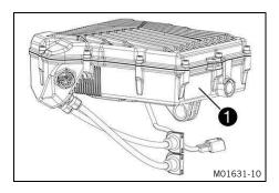
The battery identification number (**BIN**) **1** is located on a sticker on the LV traction battery.
