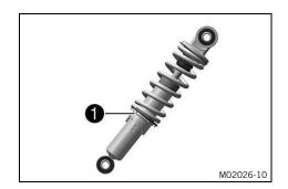
Adjust the spring preload by turning adjusting ring 1
