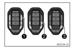
All segments 1 light up: charging level 70 % - 100%. Four segments 2 light up: charging level 50 % - 70 %. Two segments 3 light up: charging level 30 % - 50 %.
