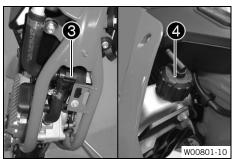
Water pump 3 in the engine circulates the coolant.
