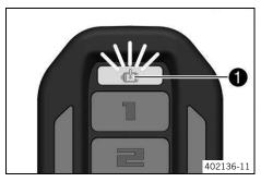
**Malfunction indicator light**The warning tones of the multifunction element sound in sync with the flashing interval of malfunction indicator light **1**.
