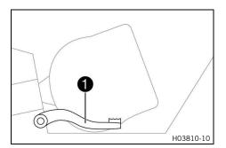
Brake pedal **1** is located in front of the right footpeg. The rear brake is operated with the brake pedal.
