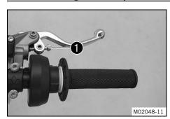
Adjust the basic position of the hand brake lever with adjusting screw 1 to the rider's hand size.
