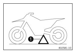
The fixture for plug-in stand **1** is located on the frame on the left side of the vehicle.
