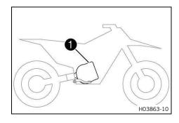
The engine number  $\P$  is located on the left side of the engine under the engine sprocket.
