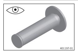
Check the hand grips on the handlebar for damage, wear, and that they are firmly seated.
