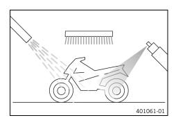
Remove the coarse dirt particles with a gentle water jet.
