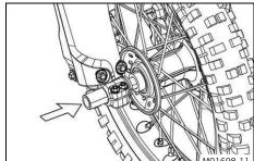
Clean and lightly grease the wheel spindle.
