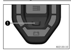
The ride mode button 1 determines the ride mode (p. 22). The ride mode button is only active if the magnetic switch under the seat [3] (p. 19) is mounted.
