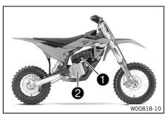
The LV traction battery **1** is air-cooled. The electric motor **2** is liquid-cooled.
