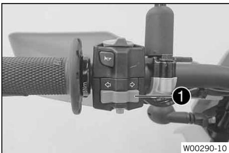
Turn signal switch ❶ is fitted on the left side of the handlebar.
