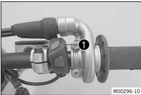
The stop button **1** is located on the right side of the handlebar.
