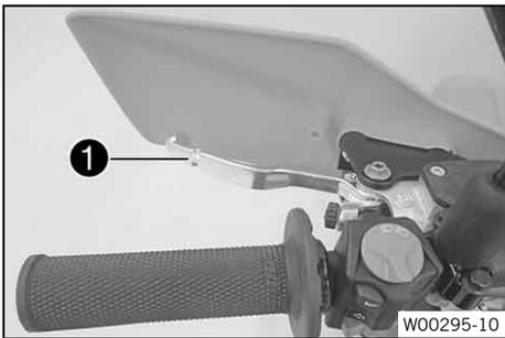
Clutch lever ❶ is fitted on the handlebar on the left. The clutch is activated hydraulically and adjusts itself automatically.
