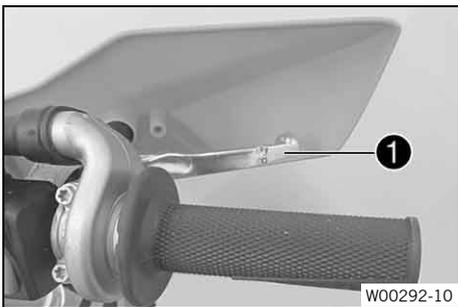
Hand brake lever ❶ is fitted on the right side of the handlebar. The front brake is engaged using the hand brake lever.
