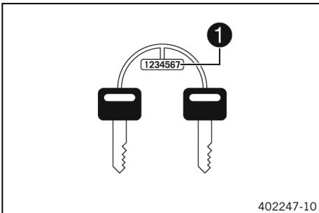
The key number **1** for the steering lock is stamped onto the key connector.
