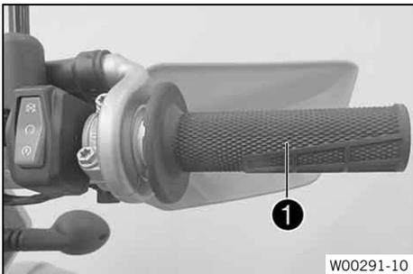
Throttle grip ❶ is fitted on the right side of the handlebar.
