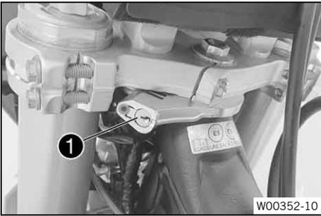
Steering lock ① is fitted on the left side of the steering head. The steering lock is used to lock the steering. Steering, and therefore riding, is no longer possible.
