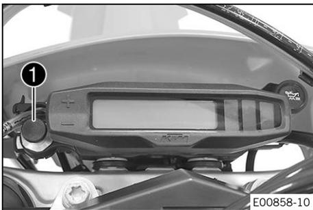
The light switch ❶ is located to the left of the combination instrument.
