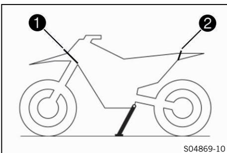
The supporting straps are located at the front **1** and rear **2** of the vehicle.
