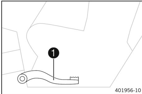
Foot brake lever **1** is located in front of the right footrest.
