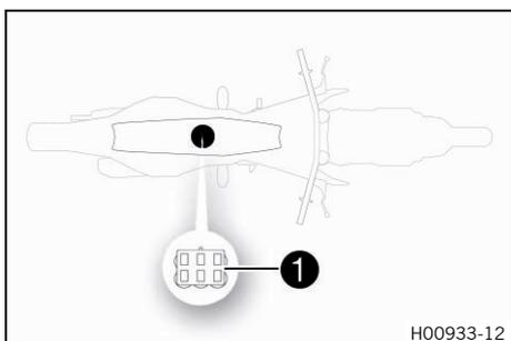
Diagnostics connector **1** is located under the seat below the engine control unit.
