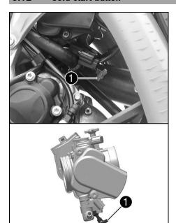
The cold start button is fitted to the bottom of the throttle valve body
