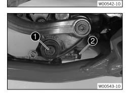
Mount and tighten screw plug with the O-ring.
