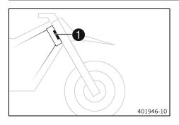
The steering head label 1 is attached to the front of the steering head.
