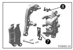
Check that spring plate in the brake caliper and brake pad sliding plate in the brake caliper bracket are seated correctly.
