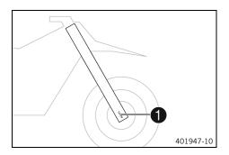
The fork article number 1 is stamped on the inside of the axle clamp.
