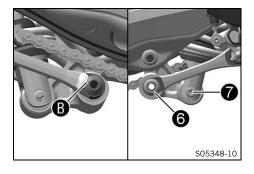
Position the foot brake cylinder.
