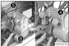
Insert the new brake linings, insert pin 6, and mount cotter pins 4.
