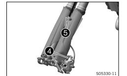
Position the brake caliper. Mount and tighten screws 4.
