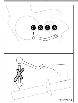
When the  $\underline{\text{quickshifter}}$  is activated, you can shift up without actuating the clutch.
