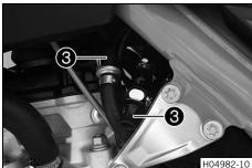
Disconnect the quick release coupling.
