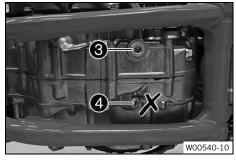
Remove oil drain plug 3 with the magnet and seal ring.
