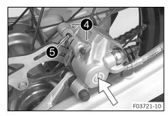
Manually press the brake caliper toward the brake disc to push back the brake piston. Ensure that brake fluid does not flow out of the brake fluid reservoir; extract some if necessary.
