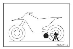
The support for plug-in stand 1 is the left side of the wheel spin-dle
