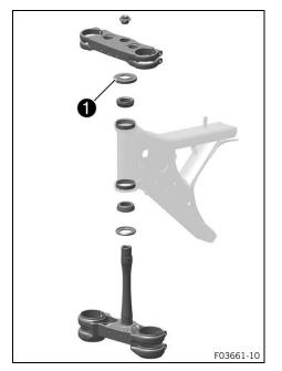
Clean the bearing and sealing elements, check for damage, and grease.
