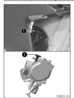
The idle setting of the throttle valve body substantially influences the vehicle's starting behavior, a stable idle speed, and the vehicle's response when the throttle is opened.
