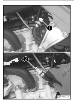
Clean quick release coupling 1 thoroughly with compressed
