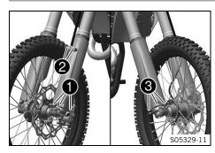
Position the fork protector on left fork leg. Mount and tighten screws 1.
