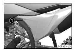
The air filter box cover is secured.
