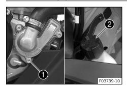
Water pump 1 in the engine circulates the coolant.
