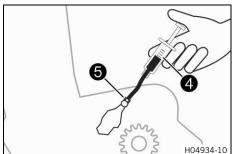
Fill bleeding syringe 4 with the appropriate hydraulic fluid.
