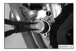
Pull oil filter out of the oil filter housing.
