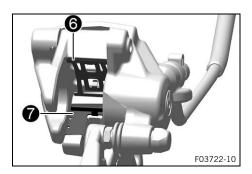
Check that spring plate 6 in the brake caliper and brake pad sliding plate 7 in the brake caliper bracket are seated correctly.
