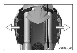
Pull both spoilers laterally off the radiator and lift off the fuel tank.
