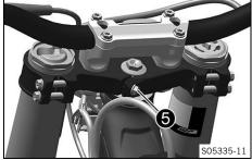
Screw, top M8 20 Nm (14.8 lbf ft) steering stem Loctite®243™
