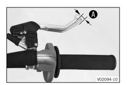
Push the handbrake lever forwards and check play **A**.
