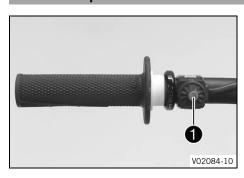
The stop button **1** is fitted on the left side of the handlebar.
