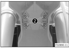
Position front fender. Mount and tighten screws 2.
