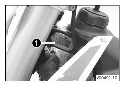
The service hour counter ① is fitted on the left side of the frame. It shows the total number of service hours of the engine. The service hour counter begins counting when the engine is started and stops when the engine is switched off.
