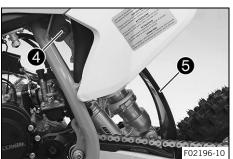
Remove screw 4, push splash protector 5 to the side, and remove the shock absorber.
