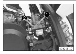
Screw in idle air adjusting screw 2 all the way and turn it to the specified basic setting.
