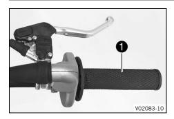
Throttle grip **1** is fitted on the right side of the handlebar.
