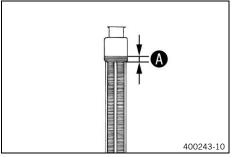
Check the coolant level in the radiator.
