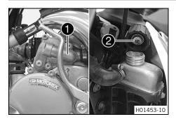
The water pump 1 in the engine forces the coolant to flow. The pressure resulting from the warming of the cooling system is regulated by a valve in the radiator cap 2. This ensures that operating the vehicle at the specified coolant temperature will not result in a risk of malfunctions.
