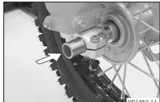
Clean and grease the wheel spindle.
