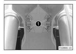
Remove screws 1. Take off the front fender.
