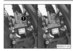
Choke **1** is fitted on the left side of the carburetor. Activating the choke function frees a drill hole in the carburetor through which the engine can draw extra fuel. This results in a richer fuel-air mixture, which is needed for a cold start.
