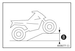
Move the vehicle into the position shown and secure it against rolling away. Height difference must be reached.
