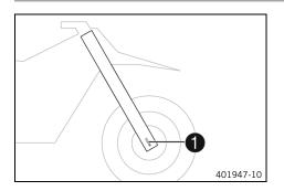
The fork article number **1** is stamped on the outside of the axle clamp.
