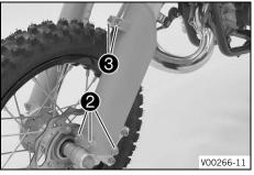
Position fork protector on left fork leg. Mount and tighten screws 2.
