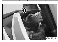
Turn the oil tank cap 1 counterclockwise and pull it up.
