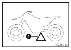
The fixture for plug-in stand **1** is located on the frame on the left side of the vehicle.
