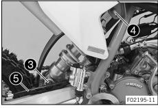
Raise the link fork, mount and tighten the shock absorber with screw 3.
