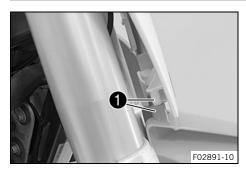
Position the fender with drill holes
