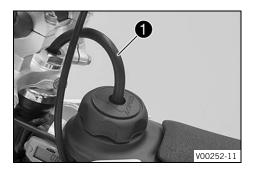
Mount the fuel tank filler cap and turn it clockwise until the fuel tank is tightly closed.
