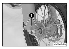
Position fork protector on the right fork leg. Mount and tighten screws 1.
