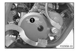
Mount and tighten plug with a new seal ring.
