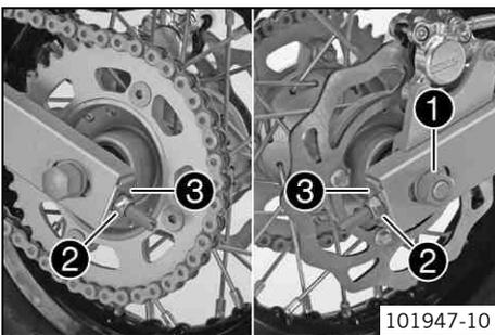
**11.35 Checking the chain, rear sprocket, engine sprocket and chain guide**
