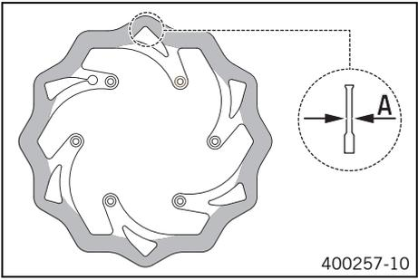
– Check the thickness of the front and rear brake discs at several places on the disc to see if it conforms to measurement **A**.
