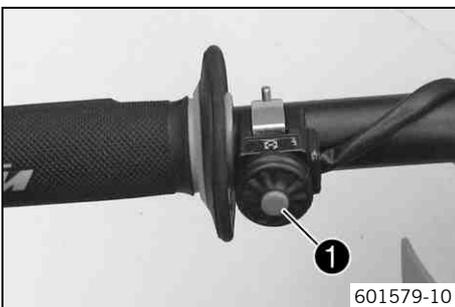
Kill switch ❶ is fitted on the left side of the handlebar.
