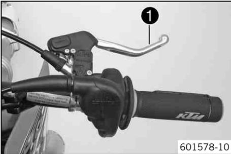
Hand brake lever ❶ is fitted on the right side of the handlebar. The hand brake lever is used to activate the front brake.
