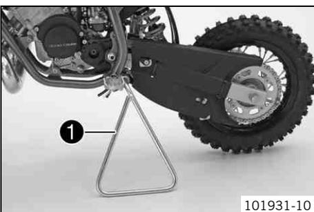
The fixture for the plug-in stand ❶ is located on the frame on the left side of the vehicle. The plug-in stand is used to park the motorcycle.
