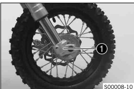
The fork part number ❶ is stamped on the outside of the axle clamp.
