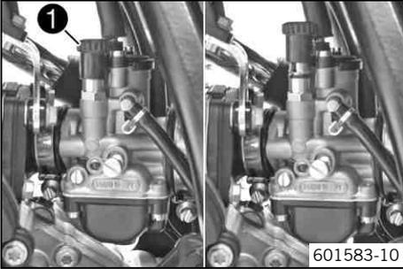
The choke knob ❶ is fitted on the left of the carburetor. Activating the choke function frees an opening through which the engine can draw extra fuel. This results in a richer fuel-air mixture, which is needed for a cold start.
