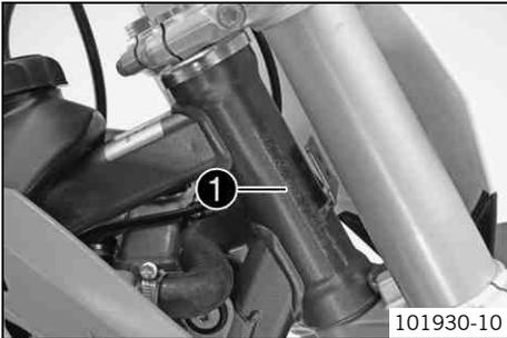
The chassis number ❶ is stamped on right of the steering head.
