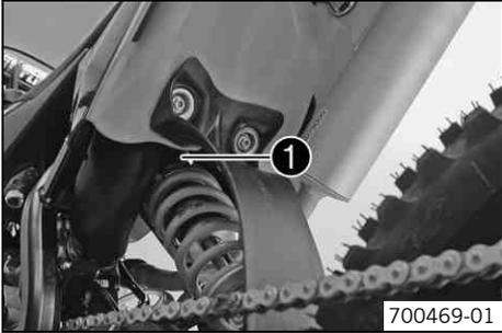
The shock absorber part number ❶ is stamped on the top of the shock absorber above the adjusting ring towards the rear.
