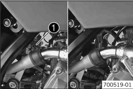
The choke lever ❶ is fitted on the right of the carburetor. Activating the choke function frees an opening through which the engine can draw extra fuel. This results in a richer fuel-air mixture, which is needed for a cold start.
