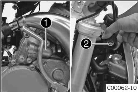
The water pump ❶ in the engine forces the coolant to flow. The pressure resulting from the warming of the cooling system is regulated by a valve in the radiator cap ❷. This ensures that operating the vehicle at the specified coolant temperature will not result in a risk of malfunctions.
