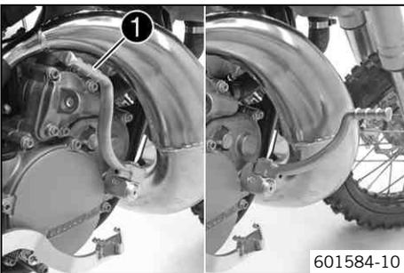
The kickstarter ❶ is fitted on the right of the engine. The kickstarter can be swiveled.
