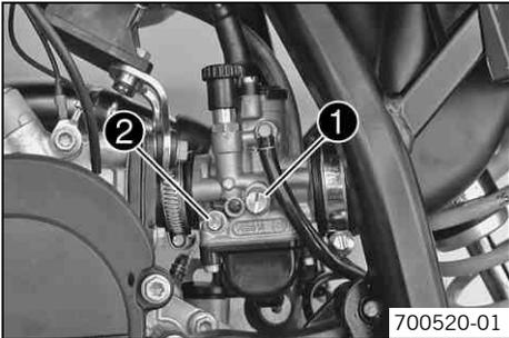
The idle setting of the carburetor has a big influence on the starting behavior, stable idling and the response to throttle opening. That means that an engine with a correctly set idle speed is easier to start than if the idle is set wrongly.
